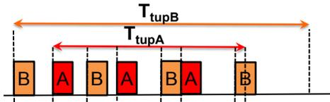
Fig. 2. Synchronization in RA-TDMA round, with 2 concurrent RA-TDMA rounds
