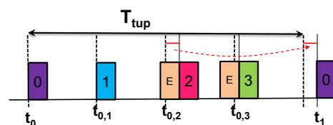
Fig. 1. Synchronization in RA-TDMA round, with external traffic
