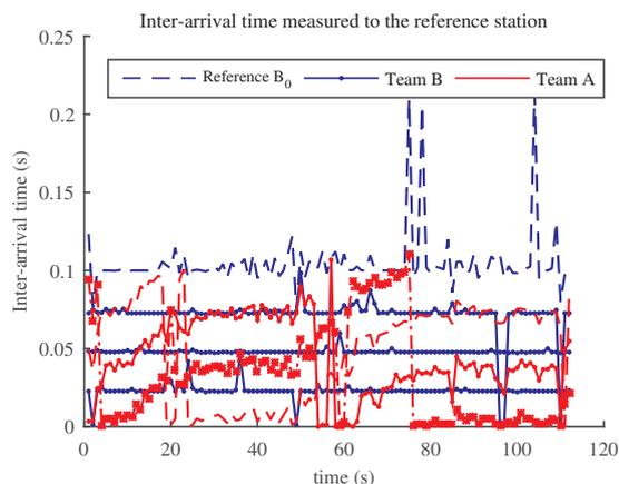
Fig. 7. Time offsets of both teams receptions (A and B) measured by the reference node of Team B
